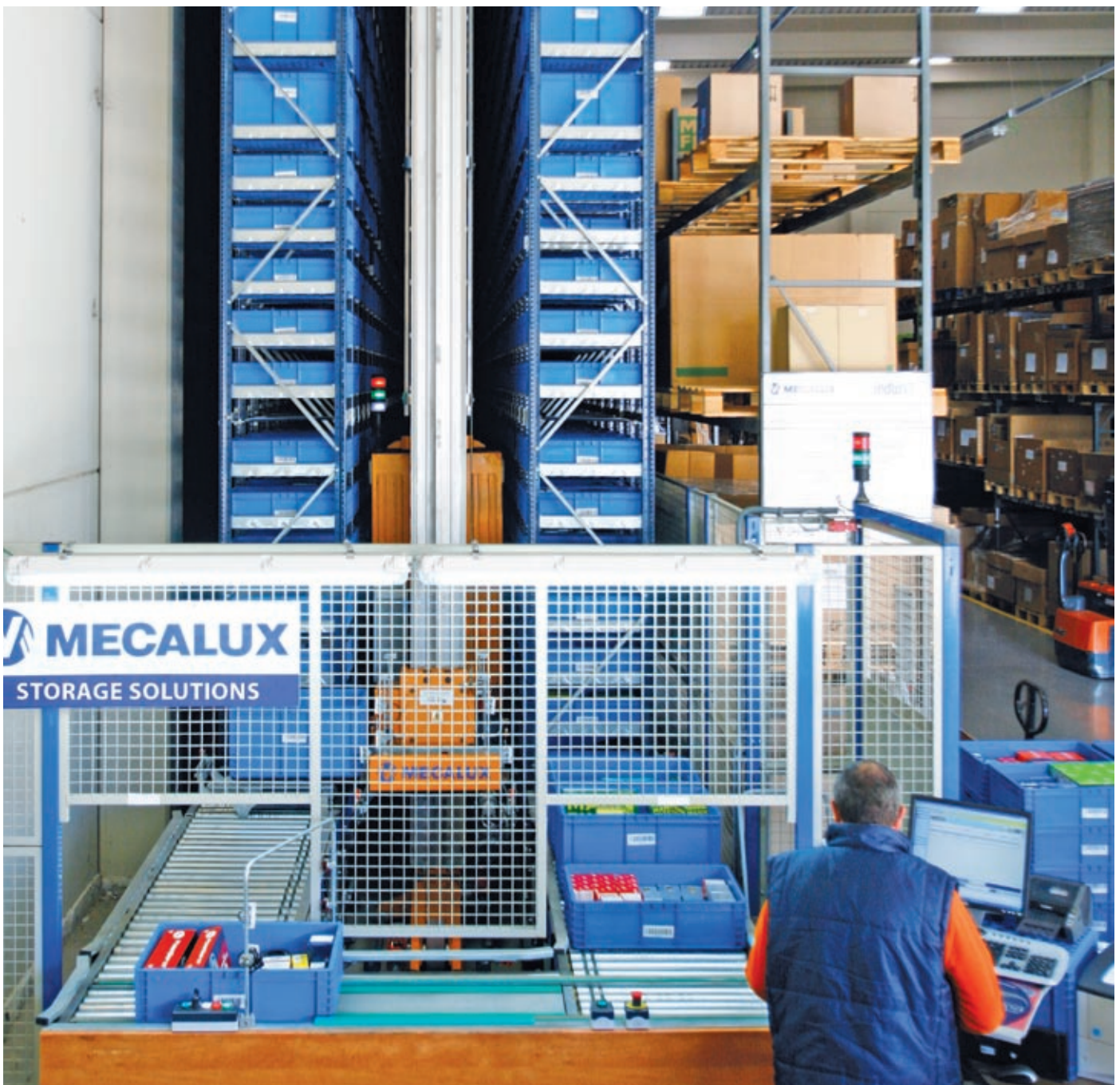
Detail of Front Picking Station with Single Head-End and Dual Extractor Pole
