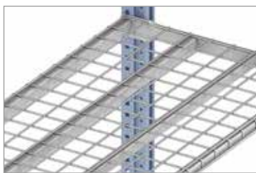
Detail of cross ties
